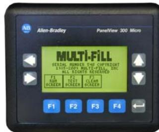
A small Allen Bradley PanelView graphics terminal provides a user friendly interface to the PLC for set-ups with production, test, and clean modes. With less moving parts, adjustments can be done while the machine is operating and maintenance is reduced.
