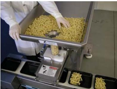
Product is loaded into the top pan and manually fed to the filling tube by an operator.
